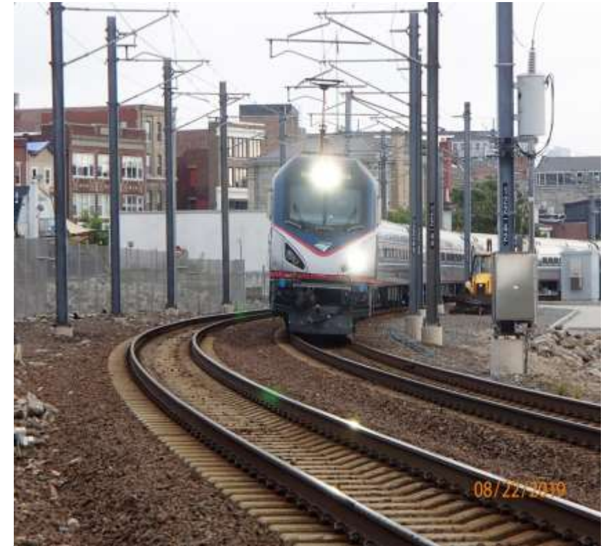
Catenary wires are under constant tension
