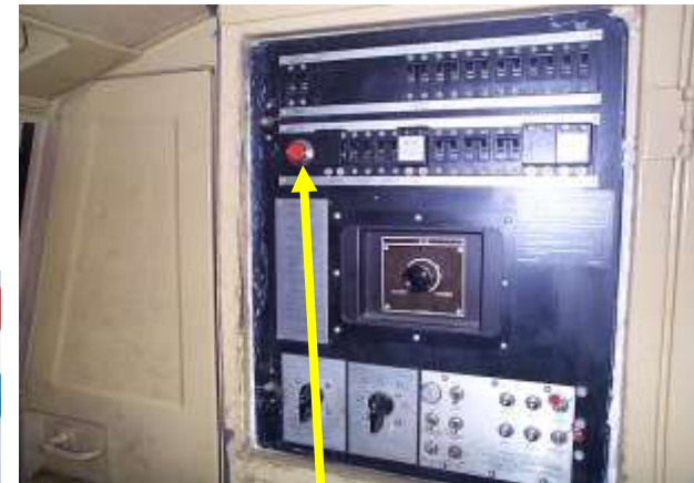
Emergency fuel Trip (shut off) on the panel on the rear wall of the engineers compartment
